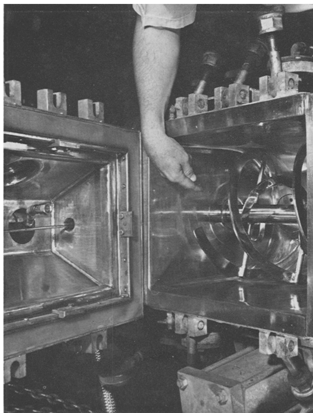
FIG. 3. Reactor for ammoniation of crambe meal at atmospheric pressure.
